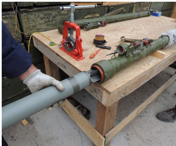
Manual disposal of Strela 2M and the inert gripstocks
