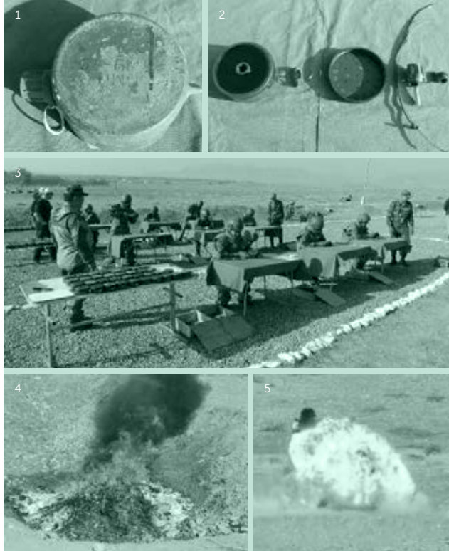
1|2 PMN antipersonnel landmine disposed with reverse engineering method; 3| Disposal of PMN antipersonnel landmines in Kyrgyz Republic, using reverse engineering method; 4| Mine parts destroyed with open burning; 5| Destruction of MON-50 antipersonnel landmines with open detonation
