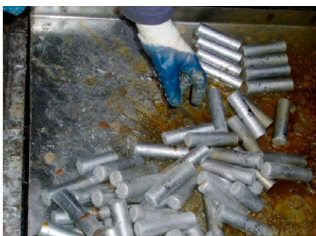
REMOVED EXPLOSIVE FROM PROJECTILE, SILVER IN COLOR INDICATES PRESENCE OF ALUMINUM
