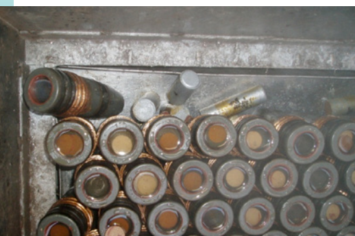
57 MM PROJECTILE INSIDE THE STEAMING CHAMBER: EXPLOSIVE BECOMES SOFT AND CAN BE EASILY REMOVED FROM THE SHELL
